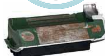
Insulated motor winding cross section
